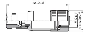
Mating connector suitable for K24 4-pole, M12 x 1 with screw connection, cable gland Pg 9, angled. Housing rotatable by  $4\times90^\circ$  in relation to the contact insert.
