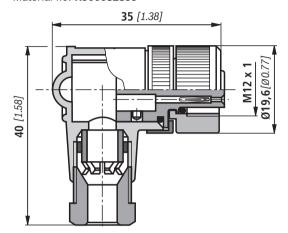
Mating connector suitable for K24-3m 4-pole, M12 x 1 with potted-in PVC cable, 3 m long.
