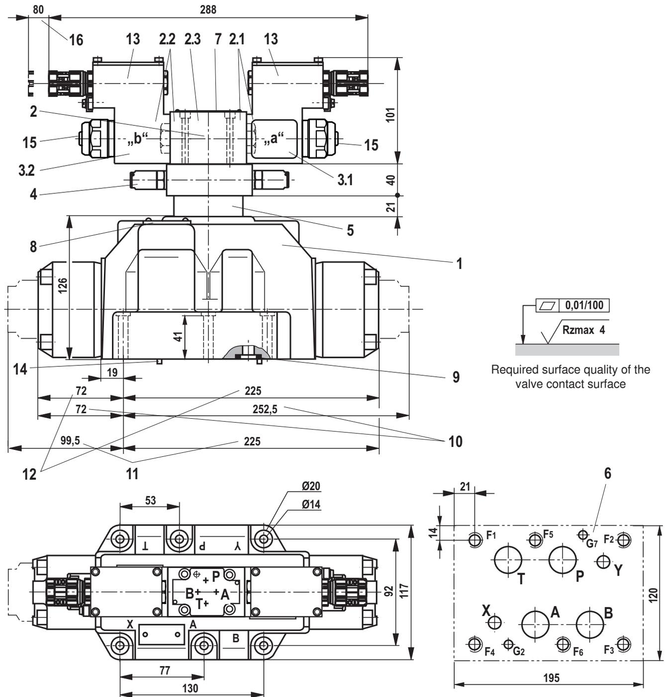
**Subplates** (separate order) with porting pattern according to ISO 4401-08-08-0-05, see data sheet 45100.
