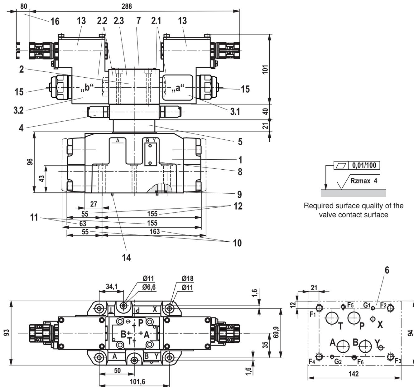
**Subplates** (separate order) with porting pattern according to ISO 4401-07-07-0-05, see data sheet 45100.
