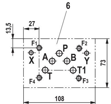
**Subplates** (separate order) with porting pattern according to ISO 4401-05-05-0-05, see data sheet 45100.
