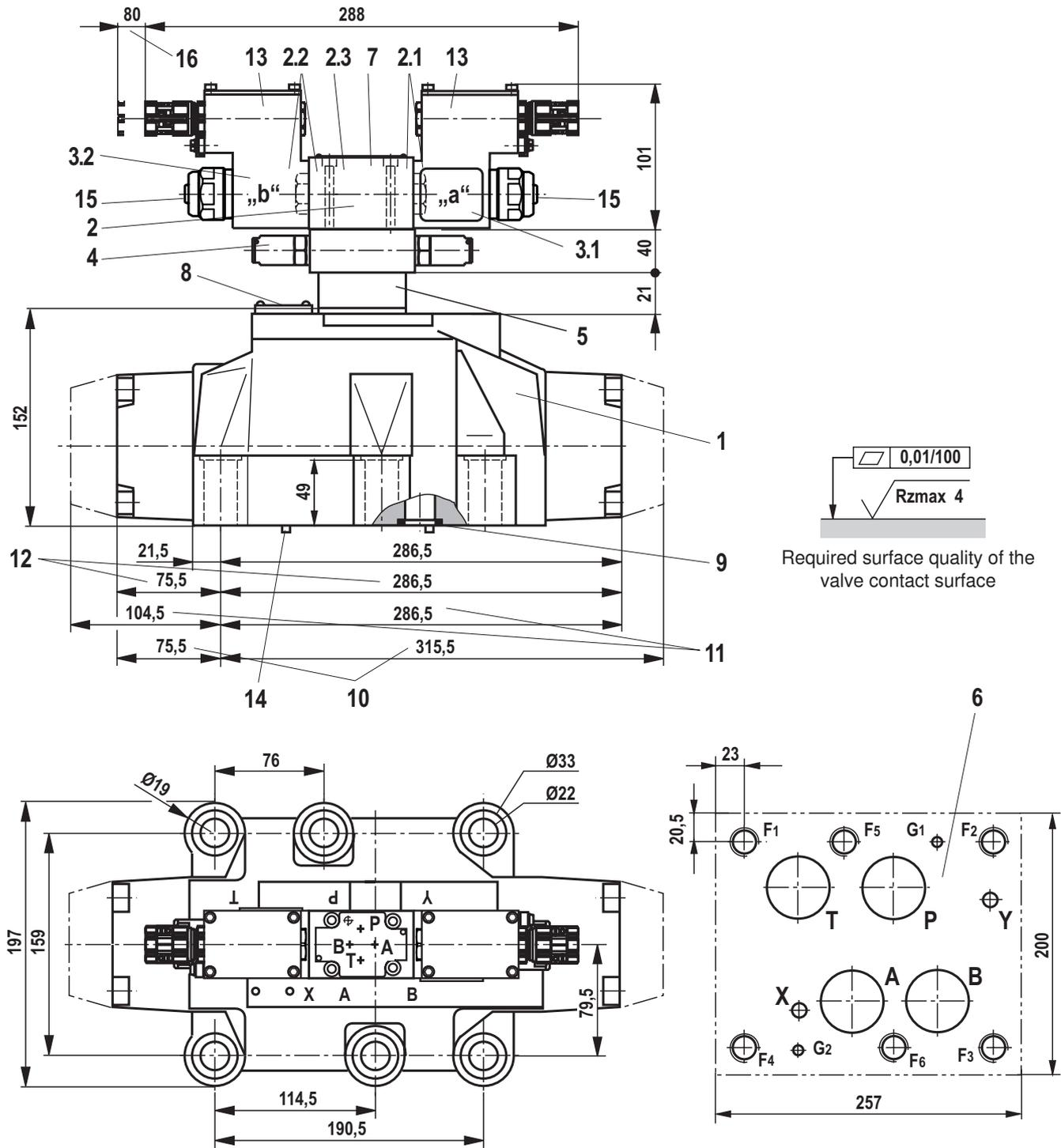
**Subplates** (separate order) with porting pattern according to ISO 4401-10-09-0-05, see data sheet 45100.
